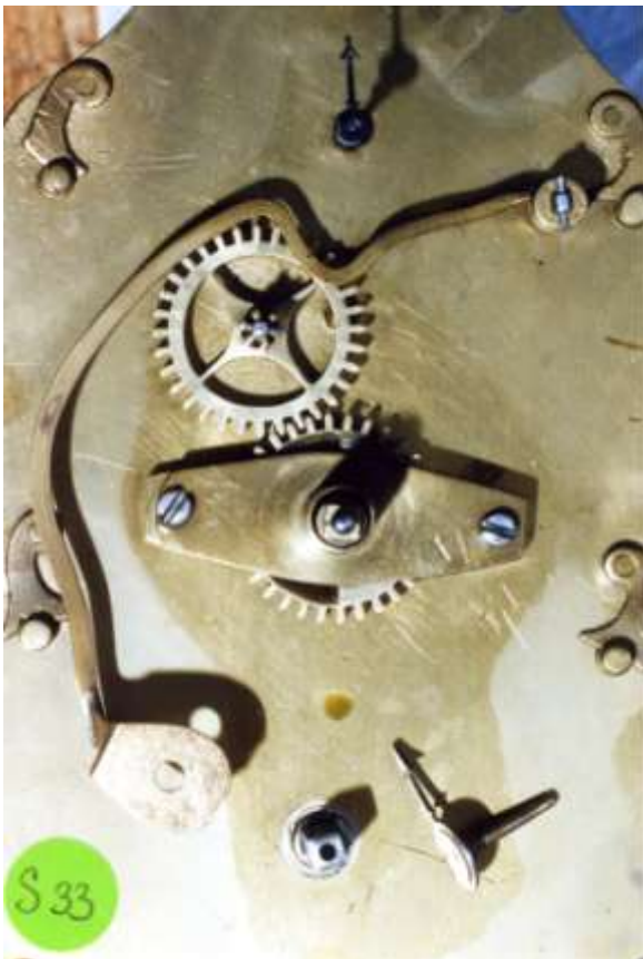
S33 Shutter "cocked", note hole in square. Thesis replaces hand with a "Tidal Elipse". Nb. unusual bridge, set on pier blocks, and cut-away to clear this curious Shutter-Arm.
