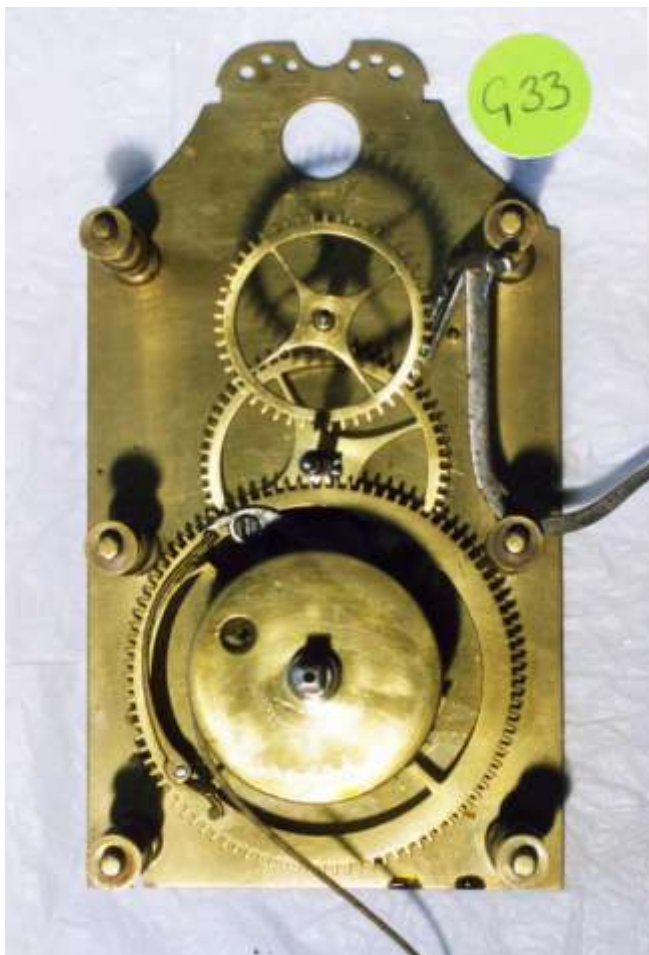
Ahasuerus Fromanteel's original form of his ' Bolt & Shutter Maintaining Power ' (B&SMP).
