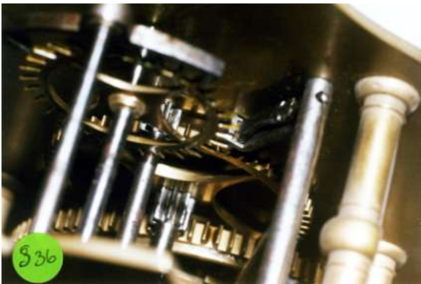
S36 Bolt of B&SMP: shown here engaged to drive the Centre-Wheel.
