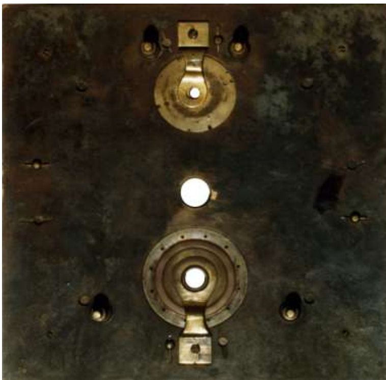
DIAL-PLATE (see composite at p.7, also pp.19-20). Constructions of Subsidiary Dials' Rotating Rings.
