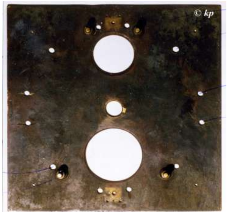
G05 DIAL-PLATE (reverse) , fittings removed.
