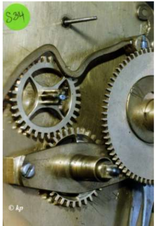
S34 Shutter arm bent under seconds arbor. Nb. 'Seconds' and Shutter Arm probably, not part of Fromanteel's original concept, having a 'verge crown-wheel' escapement.
