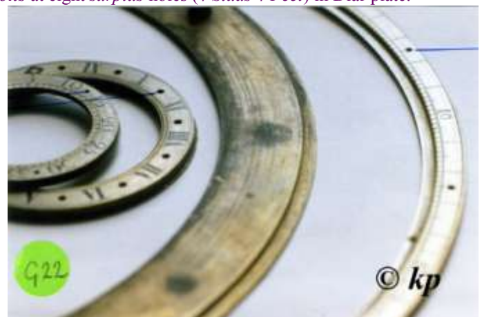
G21/G22 FIXED CHAPTER-RING: NB. Age oxidations at eight surplus holes (4 Studs 4 Feet) in Dial-plate.
