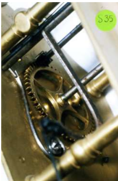
Ahasuerus Fromanteel's original form of his ' Bolt & Shutter Maintaining Power ' (B&SMP).
