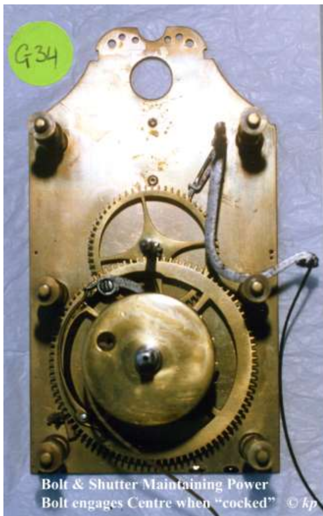
Ahasuerus Fromanteel's original form of his ' Bolt & Shutter Maintaining Power ' (B&SMP).
