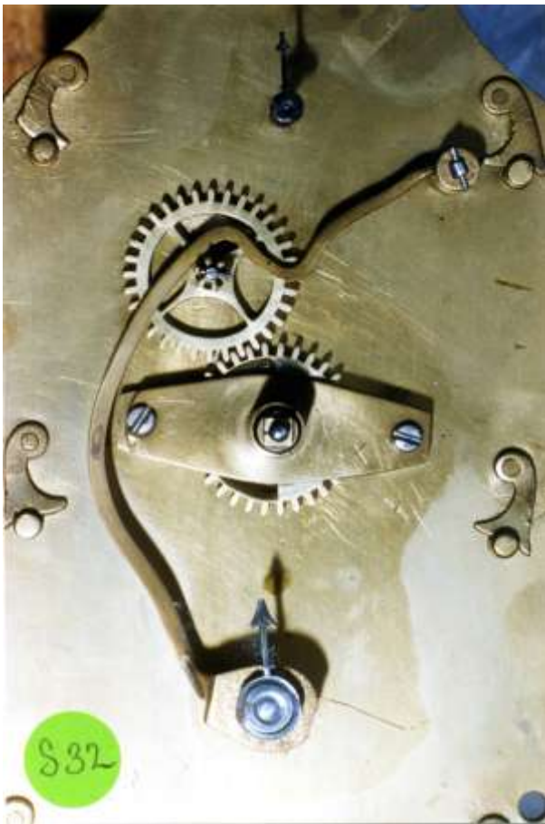
S32 Shutter Closed and Locked by the Hour-Hand
