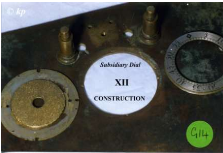
G14 360° Rotatable 'Seconds-Ring': flange behind dial, held by its Zone-Disc, supported by a Bracket.
