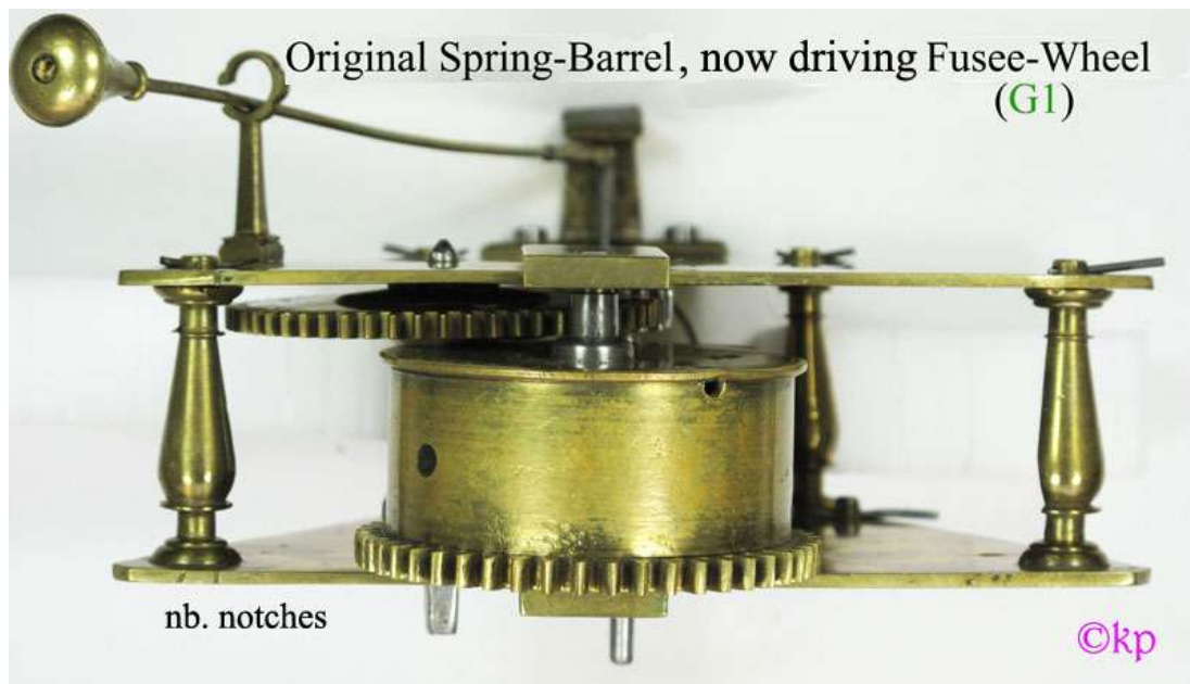
View: Original seamed Spring-Barrel, with added Great-Wheel.
