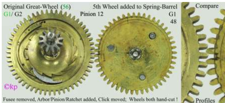
View: Original Fusee Great-Wheel, New Wheel on Spring-Barrel
