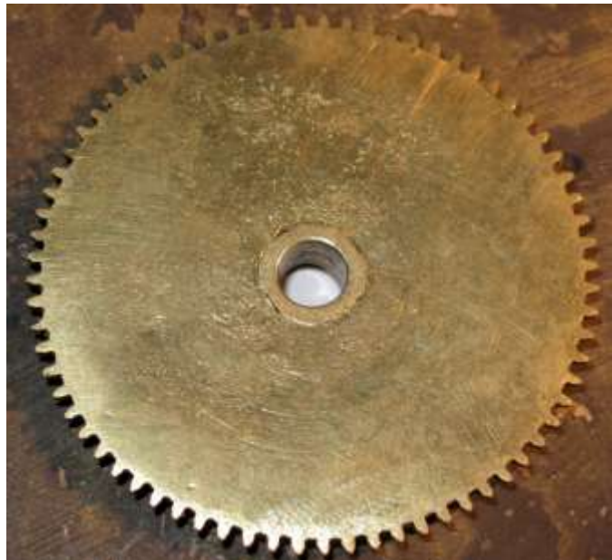
Motion-Work: Minute-Wheel 30, Reverse-Minute 30/6, Hour-Wheel 72, nb. plugged Cannon.
