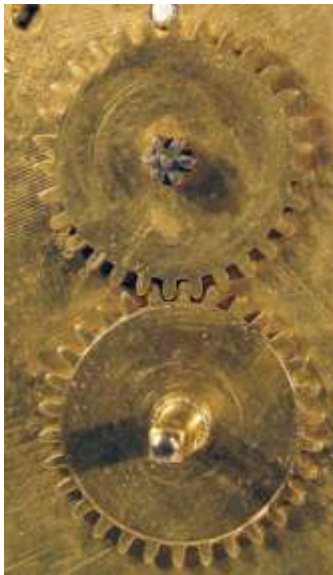
Motion-Work: Minute-Wheel 30, Reverse-Minute 30/6, Hour-Wheel 72, nb. plugged Cannon.
