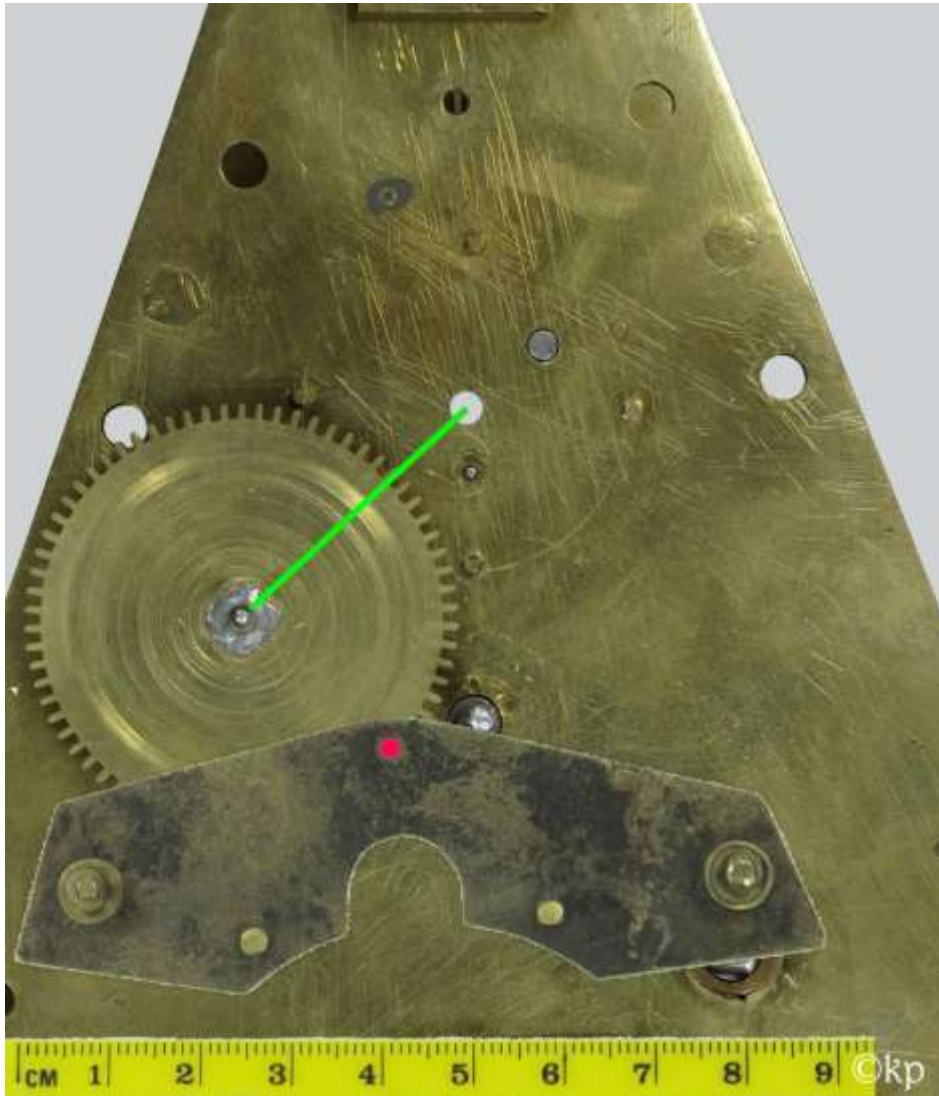
View: Reverse Minute (Rev.) Ø 4.6 cm. Pedestal Bridge (Reverse) Note 'fore-aft' Positioning Studs on Front-plate (4) and Bridge (3).
