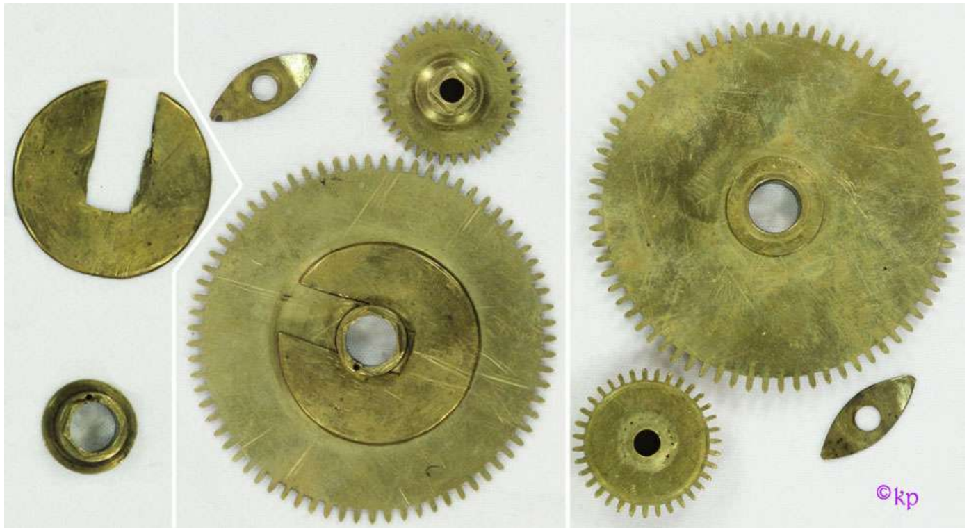
View: The Hour-Wheel (72 teeth), with Minute-Wheels of 35 teeth. Nb. Round Key-plate, Hexagonal Hour-Cannon, and Minute-Pipe, being typical of English constructions - as used by Ahasuerus Fromanteel.
