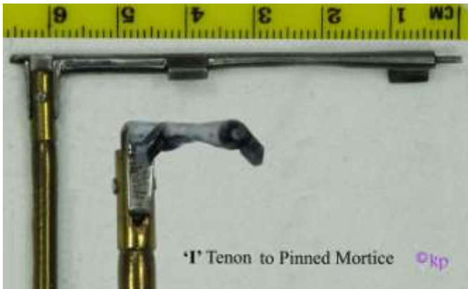
View: Pivoted-Pendulum pinned to 'I' bar of long Verge.
