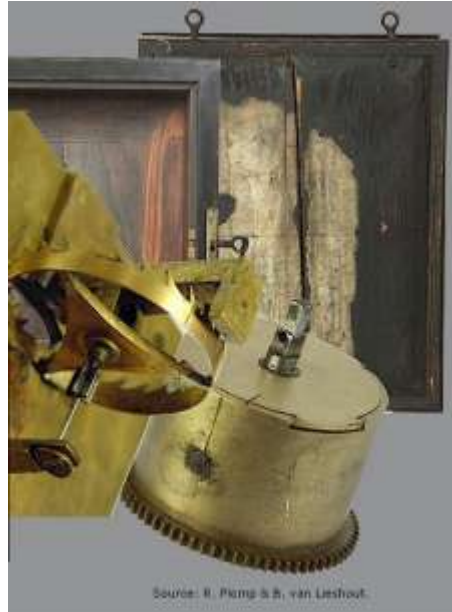
Views of exceptional dovetailed barrel-cap by courtesy of Berry van Lieshout and Dr Reinier Plomp. Hour hand as advertised at discovery.
