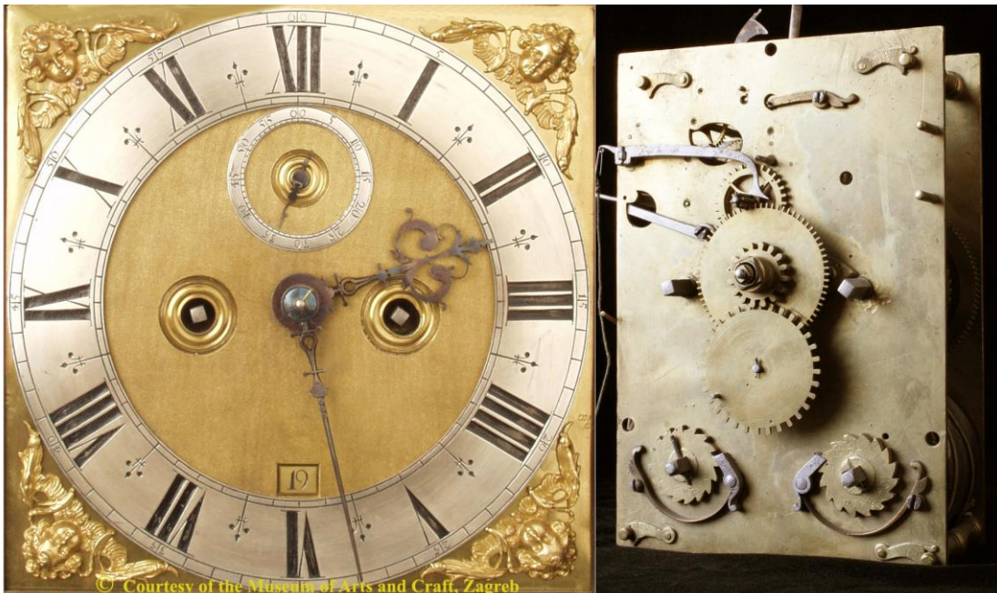
Dial of a rare fusee-clock showing the Seconds, by 'A=Fromanteel Hage' a previously unknown Fromanteel address, ( KP ). The fine original hands are typical of the Fromanteel-Clement workshops. Distorted ring by wear at Fusee pivots- note 'bumped' pivot. The movement has Fromanteel's original pivoted-pendulum to early 'Tic-Tac' escapement with his knife-edge suspension and steel keeper, and having typical English Five-Wheel Trains on Fusees; circa 1680. ( RH, Part 2 . "The Seconds' Hiatus?" p.29).
