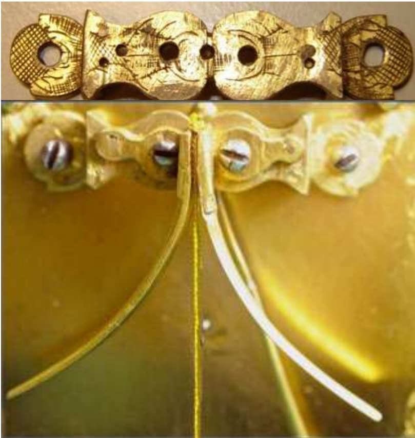
View: Treffler's Original, Engraved and Gilded, Back-Cock.
