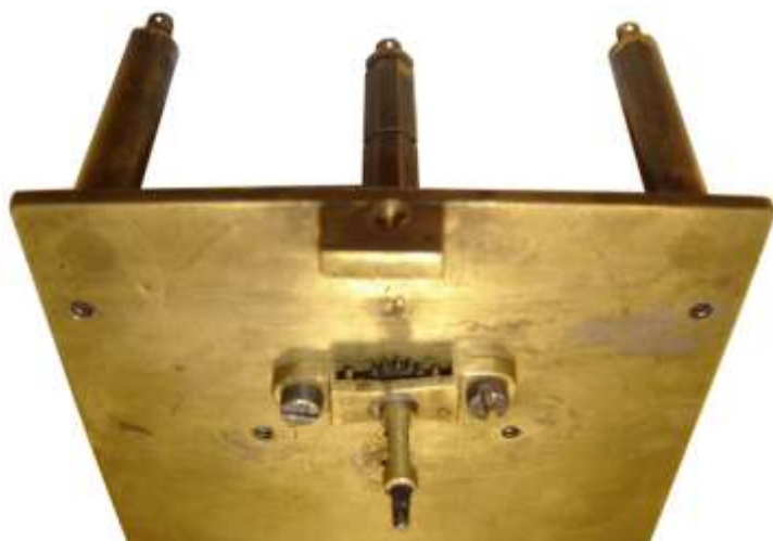
The Upper Front-Plate - Seconds' Bridge and Arbor. (The Motion-Work shown at p.5)
