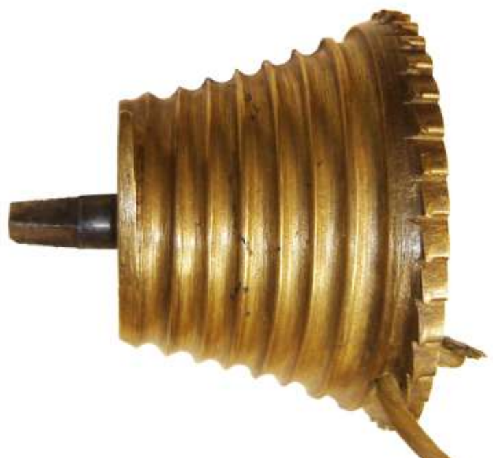
Treffler's ' Augsburg ' Fusee with Ratchet.
