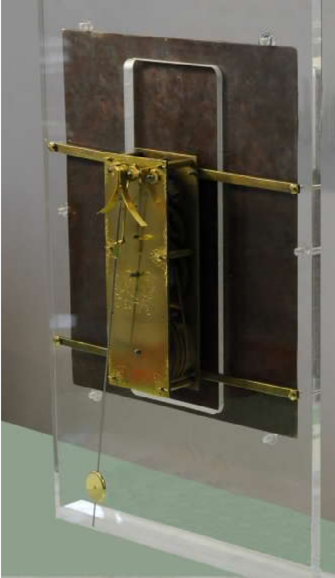
Formerly, the long straps secure the movement, with dial attached, to the door of the lost Tabernacle case.
