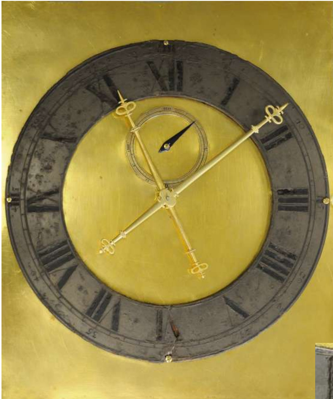
Above: " Il quadrante " Polished Gilt-Copper Rectangular Dial-plate, Pewter Chapter-Ring (distressed), Fine Counterpoised Looped Hands, replaced Silvered Seconds' Ring. Right: The Copper Dial-plate is gilded everywhere except beneath the annulus of pewter chapter-ring, thereby conserving valuable gold. [Ahasuerus Fromanteel did likewise]
