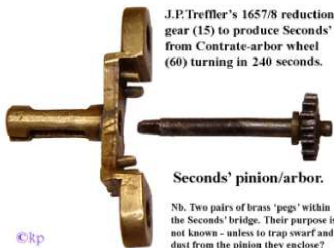
Treffler's Seconds' Reduction Gear to Convert Contrate 240 Seconds into 60 Second's at Dial.
