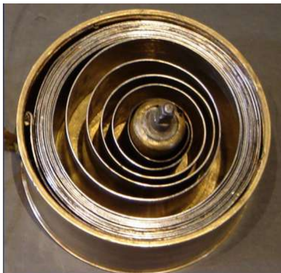
Left: The Narrow Barrel, with Long Main-Spring. "Molla e barile"
