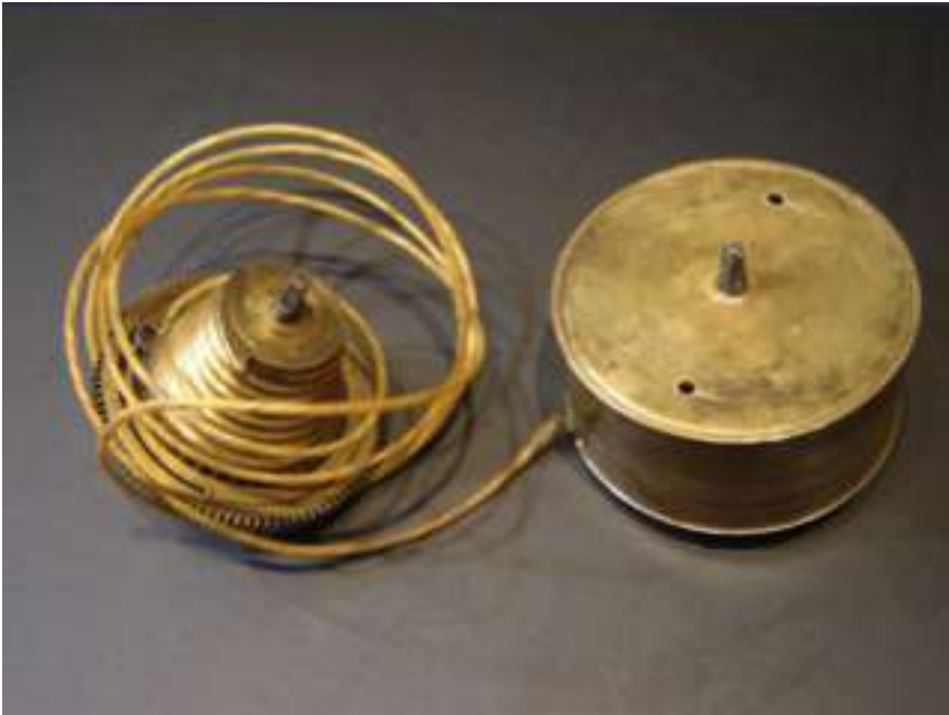
Left: The Narrow Barrel, with Long Main-Spring. "Molla e barile"
