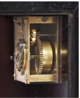
**N**ote. The remote *Alarum* is built in a like manner as the movement, it too has square pillars, external ratchet-work, set on its back-plate; both having turned ratchets and brass springs to the steel clicks, held with screws. The alarum is wound at the right face of the box, with the winding key. Compare this with the attached <u>Alarum</u> affixed to Coster **D8**, when discovered, which probably was a contemporary alarum.
