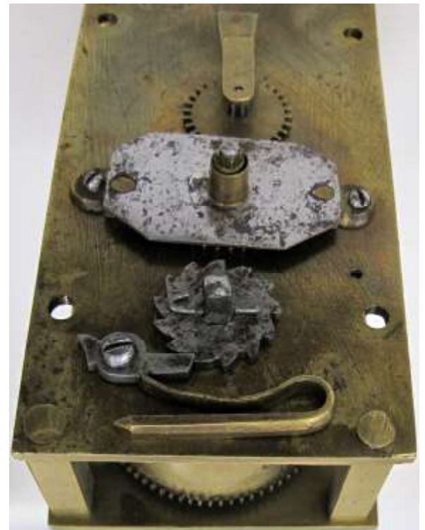
SCREWED CLICK, PEGGED SPRING, PINNED RATCHET WHEEL.
