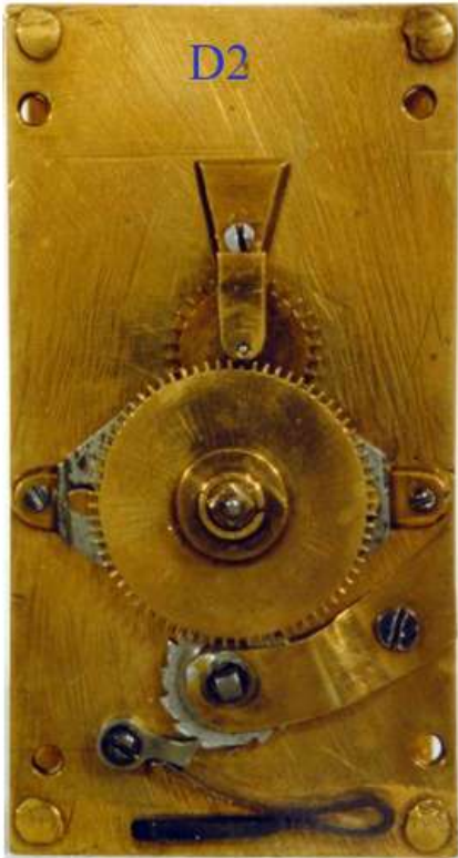
Bridge: trapezoid iron plate set on brass feet. Steel click and spring, having a brass cock to steel ratchet, vertical motion cock on wide foot.
