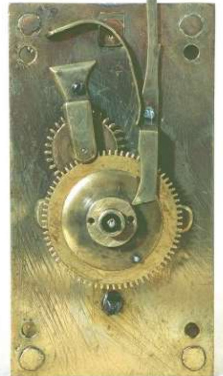
Bridge: appears to be iron plate on brass feet (cf. D1, D2, D4). The ratchet work is removed onto the back-plate. Motion cock similar to D1, but offset for alarm-work.
