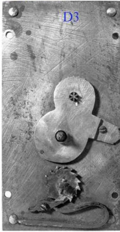
Bridge: wrought brass lobed plate, doubling as a motion cock, on a single foot. Steel click and spring, pinned ratchet. Small dial-studs and rivets.
