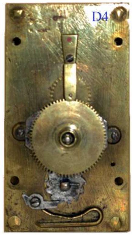
Bridge: trapezoid iron plate set on brass feet. Steel click, brass spring, pinned ratchet-wheel, vertical motion cock on a narrow foot. Nb. Red copper steady-pins are only found in D4.
