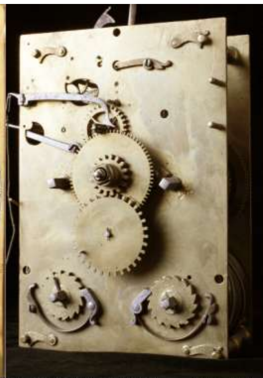
Fromanteel's typical layout: Bugle-latches; reversed ratchets and clicks (corrected by direction of line); scroll-foot to brass click-springs and long-cock for ' Tic-Tac ' arbor; Fesico shaped bridge, integral steady-pins (2nd method); ID punches ( NL, 'tekawa' ): lifting-piece with Strike re-set pull; passing half-hour strike; steel posts and port for B&SMP (Shutter set on Dial collet); shaped ports; Seconds' direct off 4th Wheel in Tic-Tac train.
