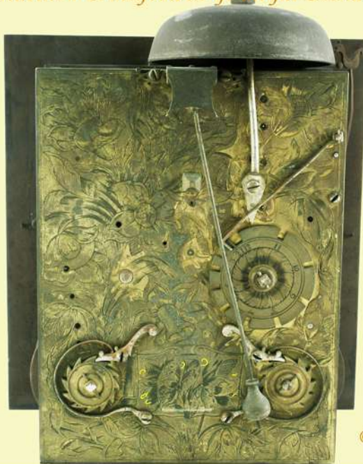
A fine early London spring movement, c.1672, apparently anonymous. This outstanding movement having many delightful features, including a superbly engraved floral back-plate and indiosyncratic set-up ratchets and clicks, marred by the later defaced Lambrequin. Carefully added flower-heads, nevertheless, left exposed engraved strokes of original Signature.
