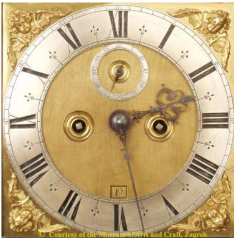
Dial of a rare fusee-clock showing the Seconds, by ' A=Fromanteel Hage ' a previously unknown Fromanteel address, ( AP ). The fine original hands are typical of the Fromanteel-Clement workshops. Distorted ring by wear at Fusee pivots- note ' bumped ' pivot. The movement has Fromanteel's original pivoted-pendulum to early ' Tic-Tac ' escapement with his knife-edge suspension and steel keeper, and having typical English Five-Wheel Trains on Fusees; circa 1680. ( RH, Part 2, "The Seconds' Hiatus?" p.29 ).
