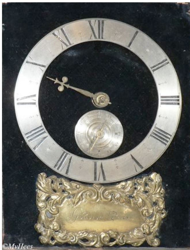
DIAL Unusual Single-Hand Display with Subsidiary Minutes and Quarter Hand turning Anti-Clockwise.
